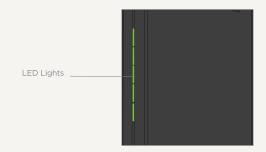
As the Modem is searching for the CLEAR 4G signal, five LED lights, located on the front of the Modem, will blink sequentially and then in unison. When the Modem is connected to the CLEAR 4G signal, the LED lights will stop blinking and remain lit.
