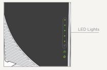
As the Modem is searching for the CLEAR 4G signal, five LED lights, located on the front of the Modem, will blink sequentially and then in unison. When the Modem is connected to the CLEAR 4G signal, the LED lights will stop blinking and remain lit.
